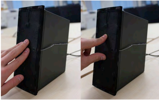
Figure 11: Volume, track-change, and fast-forward functions are controlled using finger dragging gestures.
